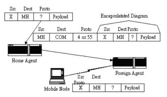
**Figure 2.2 Mobile IP Procedures**
