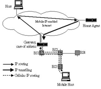
Figure 2.3 Cellular IP access Network
